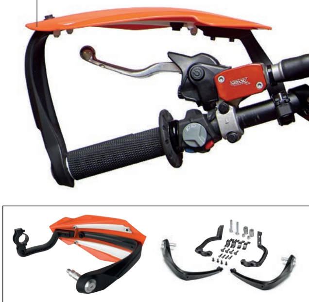
MOUNTING SYSTEM WITH HIGHLY RESISTANT PLASTIC BAR
